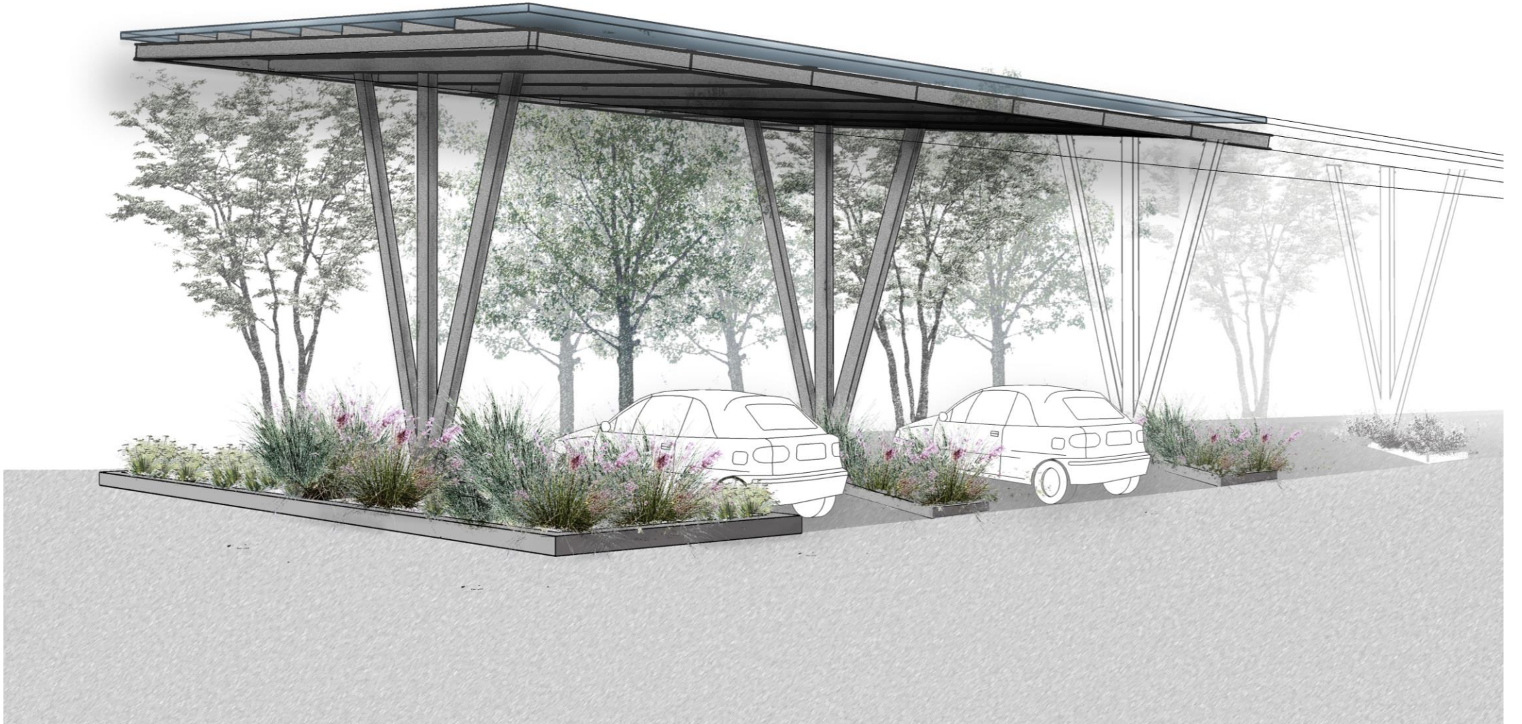
Solar Panel Support Option 2: Triple-T Post Supports
