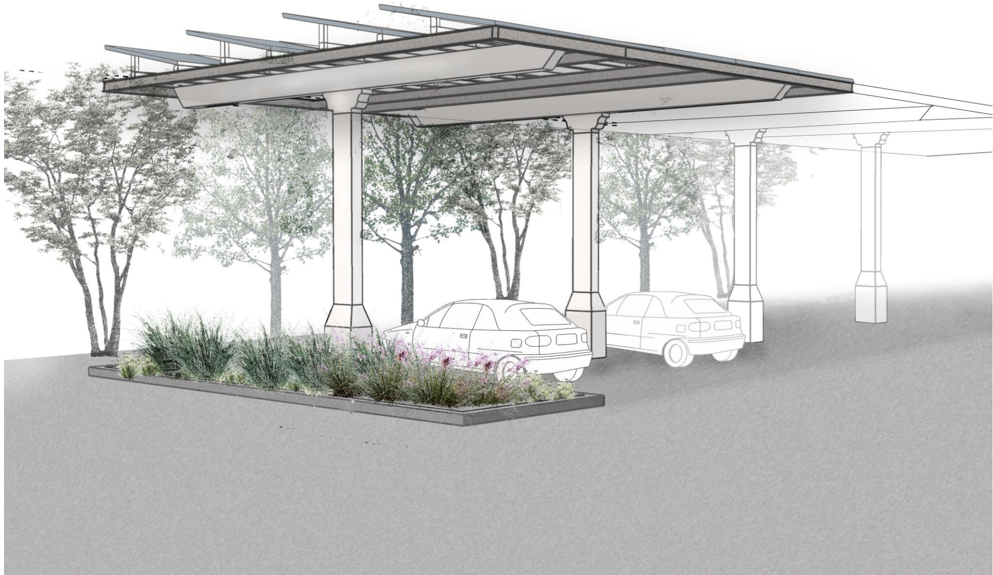
Solar Panel Support Option 3: Southwest Style T-Posts
