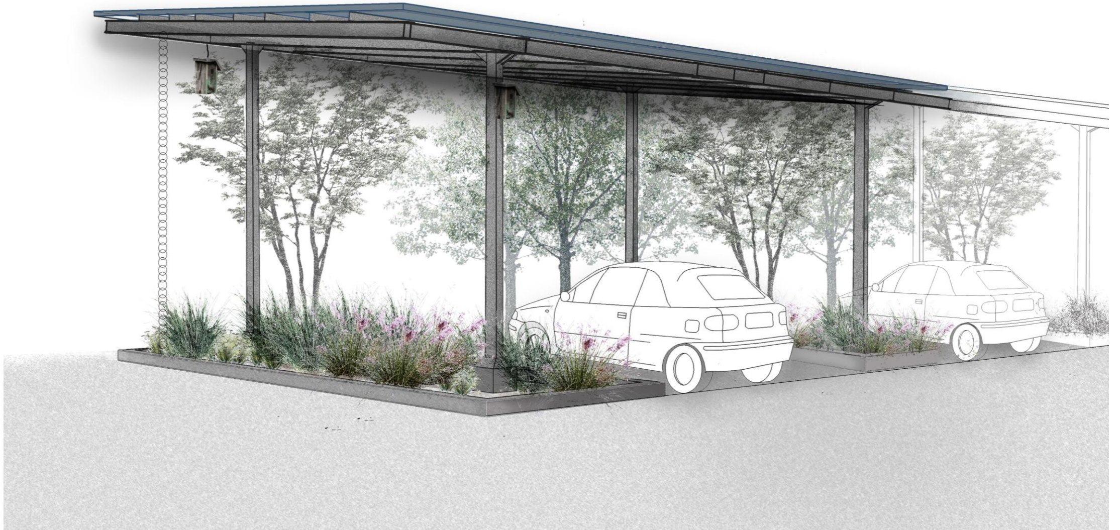
Solar Panel Support Option 1: Corner Posts
